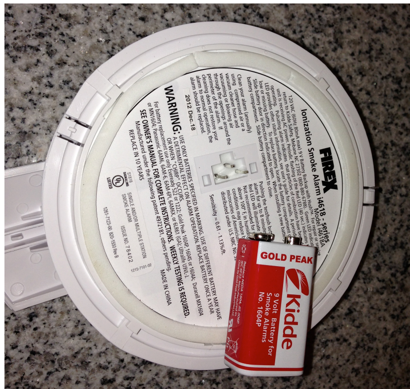
Smoke alarm with the manufacturer provided battery, and also shows manufacturer date & battery warning
